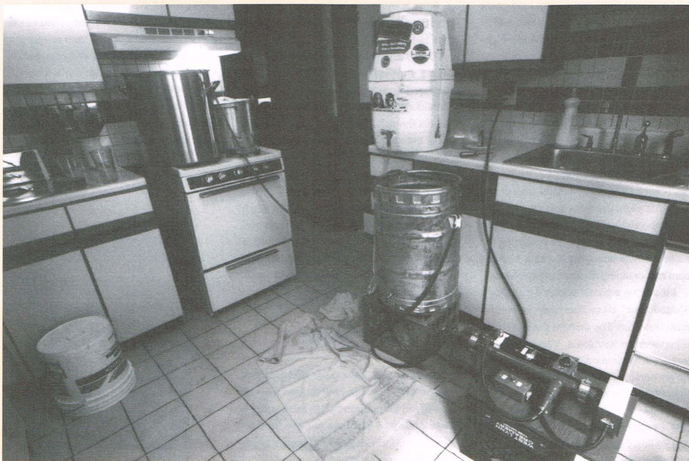
John's setup, including a stainless-steel keg that works as a mash tun with a modified Easymasher, a Little Giant pump and various other elements, all fits neatly into his brew closet when not in use.
